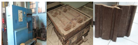
Fig 3.2 Roofing sheet material from oil palm empty fruit bunching fibers
