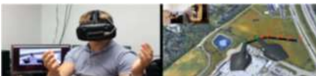
Figure 3. Set-up showing the Leap Motion device affixed onto an HTC Vive VR headset (Left). Virtual hands (on-screen) positioned in VR in place of the real user's hands (Right) [54]
